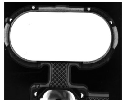
CSTG-COS5540-B Positioning for the glue of fingerprint module
