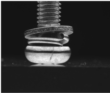
CSTG-HFS5050-W Inspection the side crack for screw
