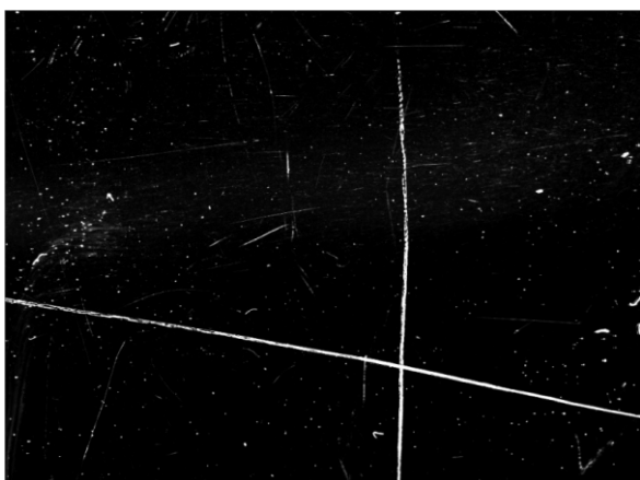
CSTG-MAS300-W 2.5d Inspection the defect of Mobile phone glass surface
