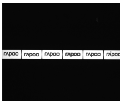
CSTG-POB20540-W Character defect inspection for key
