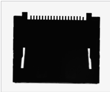
CSTG-2PFS5050-B Pin spacing inspection
