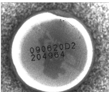
CSTG-RS9085-IR Laser engraving character inspection
