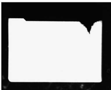
CSTG-HCOS40-R Plastic shell appearance defect inspection
