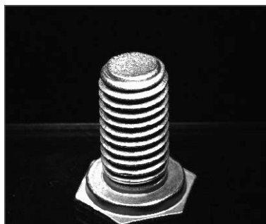
CSTG-RS7460-B Thread defect inspection
