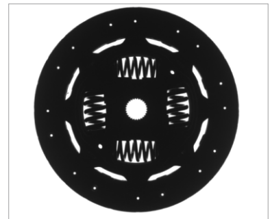
CSTG-HFS150100-W Inspection the spring of clutch plate
