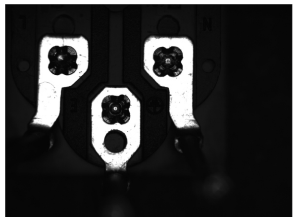
CSTG-COSC40-B Positioning inspection
