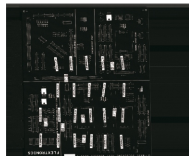
CSTG-2LPG450-R PCB board one-dimensional code inspection
