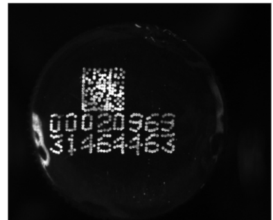
CSTG-RS7460-UV365 Bottle cap invisible RQ code inspection
