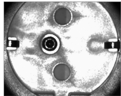
CSTG-COPS60-B Charger touch spot inspection
