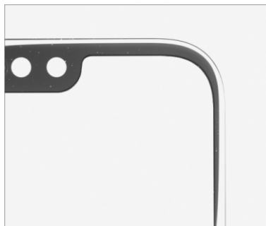
CSTG-RS7390-IR940 Phone screen AA area and ink area distance inspection
