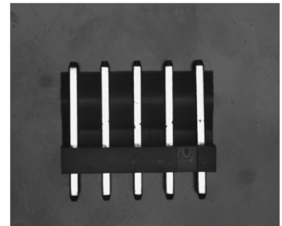
CSTG-FCS100-W Terminal pin spacing inspection
