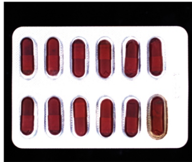
CSTG-FCS100-W Capsule leakage powder inspection
