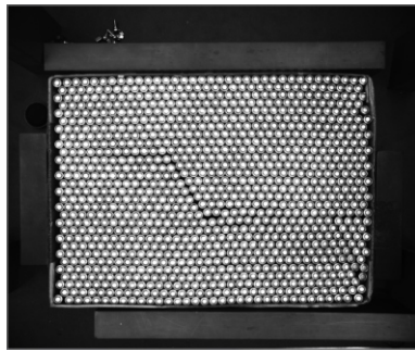
CSTG-2KFS600450Y40-W Lithium battery positioning inspection
