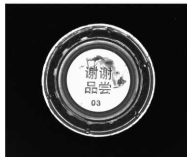
CSTG-SDS116-W Bottle cap defect inspection exposure time 4US
