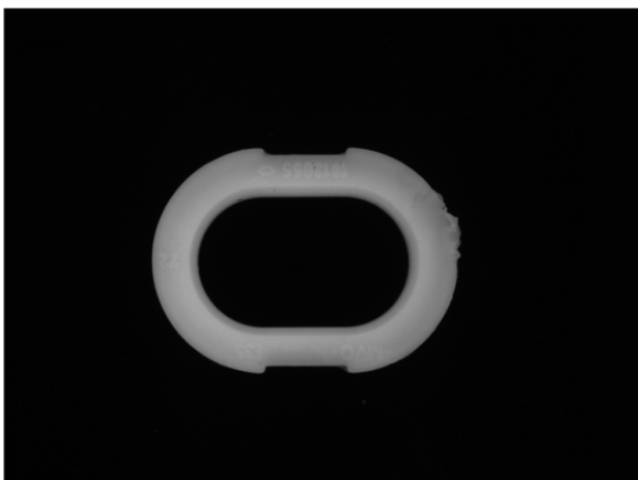
CSTG-FRS150-W Broken inspection for plastic
