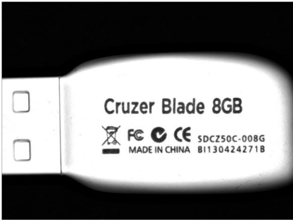
CSTG-FQS75-W Character defect inspection on USB surface
