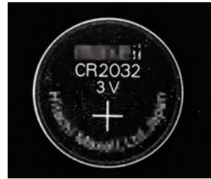
Dome Light: IDDA-KH120AW (LWD=10mm) Although the marking can be detected, the printing cannot be recognized. Dirt and contaminants on the surface are recognized.
