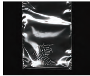
Ring Light: IMAR-200W (LWD=80mm) Halation occurs on the surface of the bag and is not ideal for quantity inspection in the plastic bag.
