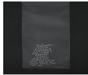
Light Used: IFHA-150W (LWD=10mm) The surface halation is reduced and internal quantity can be easily inspected.
