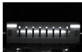
Detection of distortion of connector pins, etc.
