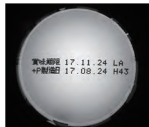
Light Used: IFHA-150W (LWD=10mm) Characters can be easily recognized due to low shadow reflection.
