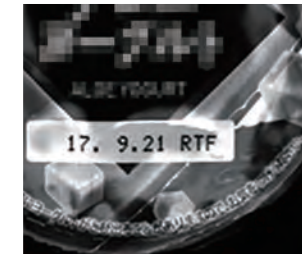
Ring Light: IMAR-130W (LWD=50mm) Color irregularity occurs on the printed area due to halation on the film surface.
