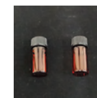
Brown bottle (Left: vegetable oil, Right: water) Body: Borosilicate glass Cap: Polypropylene
