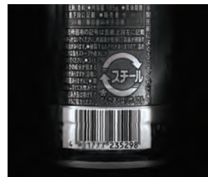
Light Used: IFHA-150W (LWD=5mm) The effect of reflections is small even on a curved surface, and the recognizable area is wide.
