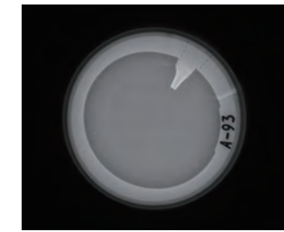
Light Used: IFHA-150IR-850 (LWD=15mm) Infrared can erase printing other than printed letters, and can recognize the printed area in addition to scratches, contamination, etc.
