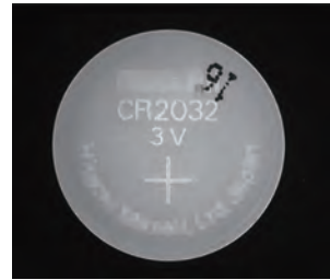
Light Used: IFHA-150W (LWD=20mm) Marking and printing can be recognized simultaneously. Dirt and contaminants on the surface are suppressed.
