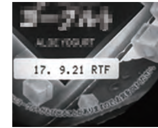
Light Used: IFHA-150W (LWD=20mm) No color irregularity due to halation, and printing and peripheral characters can be clearly recognized.
