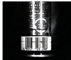
Bar Light: 2 bar lights of oblique illumination Barcodes, etc., on the curved surface cannot be recognized due to the light reflection.
