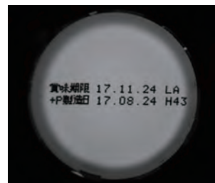
Light Used: IMAR-130W (LWD=60mm) Shadows appear around the printed area that make difficult to recognize characters
