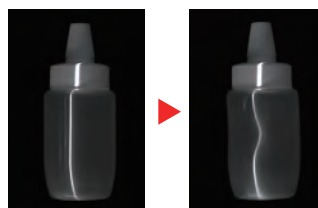
Detection of surface distortion
