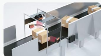
The cascade working mode allows multiple code readers to work together effectively. Subordinate code readers send their results to the master code reader, which aggregates them and outputs the final result. This simplifies the customer's application and makes managing multiple code readers easier.
